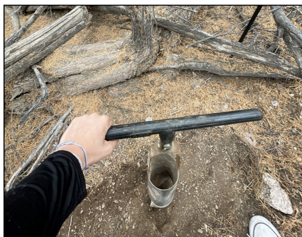
Figure C2 - Auger used to Collect Samples
