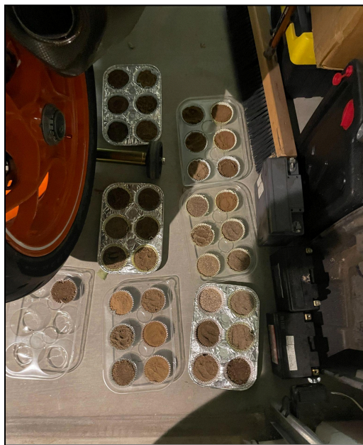
Figure C1 - Soil Drying in Disposable Tins
